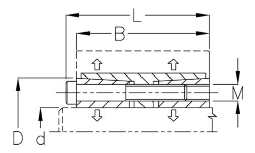
B mm = 155d H8 mm = 440D mm = 535Fit tolerance = Aksel h8, Nav H8 F kN torque = 3341.0L mm = 177M mm = M22P N/mm2 surface pressure on shaft/hub = 144 Surface roughness = R? ?  $3.2 \mu n$ T N m torque = 735000Ts N m bolt tightening torque = 930.0
